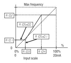
less than the R ID3 setting. When the input voltage is greater than the R ID4 ending value, the inverter outputs the ending frequency specified by R ID2.
