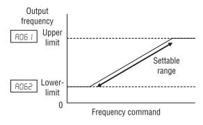
the motor or capability of the machinery. The maximum frequency setting (A004/A204) takes precedence over frequency upper limit (A061/A261).
