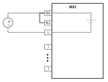
By having ability inverter doesn't block the current flowing into itself when it is not powered. This may cause the closed circuit when two or more inverters are connected to common I/O wiring as shown below to result in unexpected turning the on the input. To avoid this closed circuit, please put the diode (rated: 50 V/0.1 A) in the path as described below.
