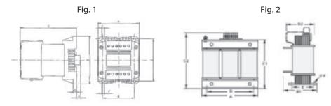
Fig. 1 (single-phase input AC reactor)
