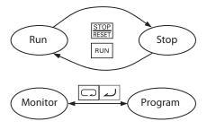
Note Some factory automation devices such as PLCs have alternative Run/Program modes; the device is in either one mode or the other. In the Omron inverter, however, Run Mode alternates with Stop Mode, and Program Mode alternates with Monitor Mode. This arrangement lets you program some value while the inverter is operating – providing flexibility for maintenance personnel.
