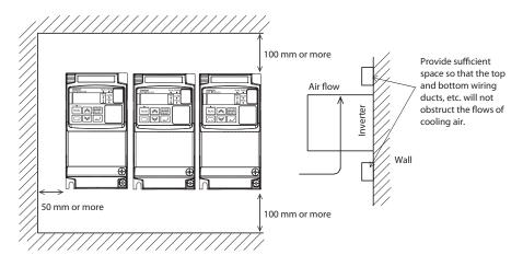
Make sure the ambient temperature remains within the rated range (-10 to 50°C). Take note that if the ambient temperature reaches or exceeds 40°C, the carrier frequency and output current must be derated (check derating tables per each inverter model in Derating Curves on page 9). If the Inverter is used in an environment exceeding the allowable operating temperature range, the product life of the Inverter (specifically, the capacitor) will be shortened.
