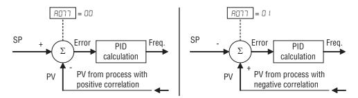
**PID deviation output** - If PID deviation " $\epsilon$ " exceeds the value in £044, output signal configured as £14 (OD) is activated.
