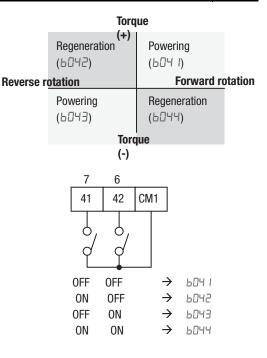
Related parameters: Over torque/under torque signal
