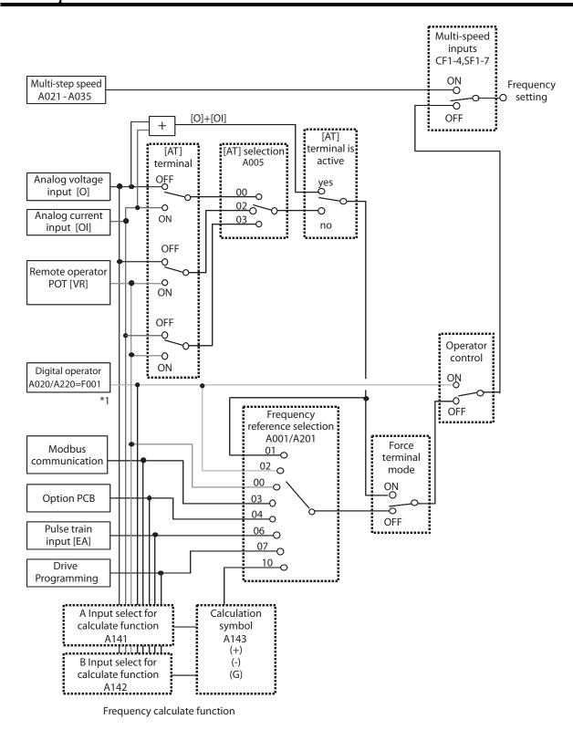
Note 1: You can set the inverter output frequency with function F001 only when you have specified "02" for the frequency source setting A001. If the setting of function A001 is other than "02", function F001 operates as the frequency command monitoring function. And by setting the frequency set in monitoring active (b163=01), you can change the inverter output frequency with function d001 or d007.
