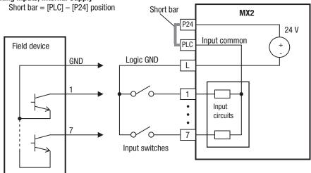
Open collector outputs, NPN transistors
