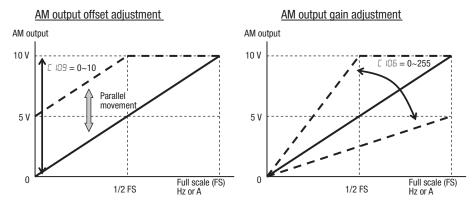
**Note** As mentioned above, first adjust the offset, and then adjust the gain. Otherwise the required performance cannot be obtained because of the parallel movement of the offset adjustment.
