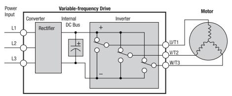
The simplified drawing of the inverter shows three double-throw switches. In Omron inverters, the switches are actually IGBTs (insulated gate bipolar transistors). Using a commutation algorithm, the microprocessor in the drive switches the IGBTs on and off at a very high speed to create the desired output waveforms. The inductance of the motor windings helps smooth out the pulses.
