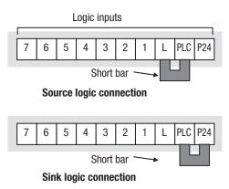
/!\ Caution Be sure to turn OFF power to the inverter before changing the short circuit bar position. Otherwise, damage to the inverter circuitry may occur.
