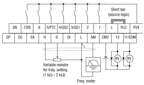
**Note** If relay is connected to intelligent output, install a diode across the relay coil (reverse-biased) in order to suppress the turn-off spike.
