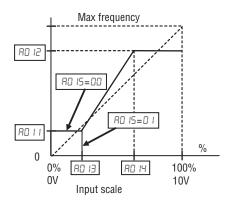
less than the RD I3 setting. When the input voltage is greater than the RD I4 ending value, the inverter outputs the ending frequency specified by RD I2.
