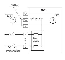
The power to the inverter control part can be supplied externally as shown below. Except driving motor, it is possible read and write the parameters by keypad and via communication even the drive itself is not powered.
