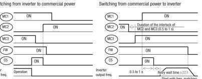
If the inverter trips because of overcurrent when it starts the motor with frequency matching, increase the retry wait time before motor starts (b003).
