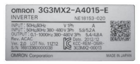
The model number for a specific inverter contains useful information about its operating characteristics. Refer to the model number legend below:
