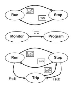
any request to run the motor is ignored. You must clear the error by pressing the Stop/Reset switch. See 6-2 Monitoring Trip Events, History, & Conditions on page 273.
