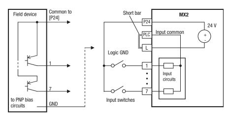
PNP transistor sousing outputs
