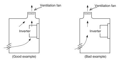
Keep the Inverter away from heating elements (such as a Braking Resistor, reactor, etc.).
