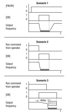
3. Scenario 3 – The Run command is applied from the operator keypad. When the [DB] terminal is ON, DC braking is applied after the delay time set by ROS3 expires. The motor is in a free-running (coasting) condition. When the [DB] terminal is OFF again, the inverter output remains OFF.
