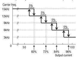
When the output current increases to 60%, 72%, 84%, or 96% of the rated current, this function reduces the carrier frequency to 12, 9, 6, or 3 kHz, respectively. This function restores the original carrier frequency when the output decreases to 5% lower than each reduction start level.
