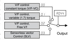
The built-in V/f curves are oriented toward developing constant torque or variable torque characteristics (see graphs below). You can select either constant torque or reduced torque V/f control.
