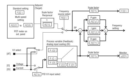
Caution Be careful not to turn PID Clear ON and reset the integrator sum when the inverter is in Run Mode (output to motor is ON). Otherwise, this could cause the motor to decelerate rapidly, resulting in a trip.
