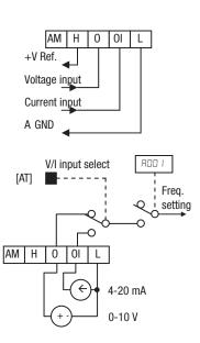
**Note** If no logic input terminal is configured for the [AT] function, then inverter recognizes that [AT]=OFF and MCU recognizes [O]+[OI] as analog input. In case either (O) or (OI) is to be refered, please ground the other.
