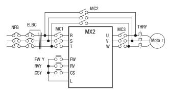
Use weak-current type relays for FWY, RVY, and CSY. The figures below show the sequence and timing of operations for reference.
