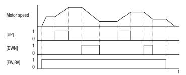
It is possible for the inverter to retain the frequency set from the [UP] and [DWN] terminals through a power loss. Parameter [10] I enables/disables the memory. If disabled, the inverter retains the last frequency before an UP/DWN adjustment. Use the [UDC] terminal to clear the memory and return to the original set output frequency.
