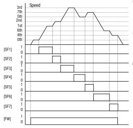
The example with eight speeds in the figure below shows how input switches configured for SF1-SF7 functions can change the motor speed in real time.
