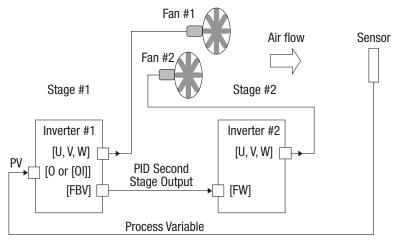
To use the PID Second Stage Output feature, you will need to choose upper and lower limits for the PV, via £053 and £052 respectively. As the timing diagram below shows, these are the thresholds Stage #1 inverter uses to turn ON or OFF Stage #2 inverter via the [FBV] output. The vertical axis units are percent (%) for the PID setpoint, and for the upper and lower limits. The output frequency, in Hz, is superimposed onto the same diagram.
