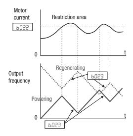
threshold for both acceleration and constant speed.
