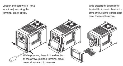
The terminal block cover is secured with one screw at the bottom right for 3.0 kW and smaller models, or with two screws on both sides for 3.7 kW and larger models.
