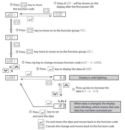
Note Function code **bxxx** are for monitor and not possible to change. Function codes **Fxxx** other than **FHHH** are reflected on the performance just after changing the data (before pressing wey), and there will be no blinking.
