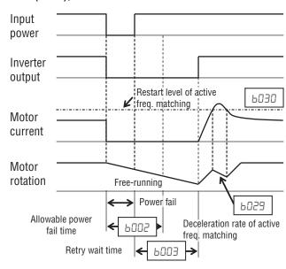
When the motor current is less than **bD3D**, the inverter increases motor speed toward the set speed. The inverter continues this retry process until the motor speed comes to the previous set speed.
