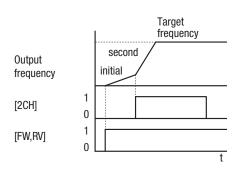
deceleration time 1). Use ROG2 (acceleration time 2) and ROG3 (deceleration time 2) to set the second stage acceleration and deceleration times.
