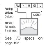
The inverter provides an analog voltage output on terminal [AM] with terminal [L] as analog GND reference. The [AM] can output inverter frequency or current output value. Note that the voltage range is 0 to +10 V (positive-going only), regardless of forward or reverse motor rotation. Use **CD28** to configure
