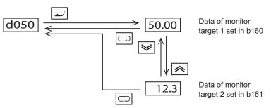
When d001/d007 Freq. set in monitoring (b163) is set to "01: Enabled", the output frequencies in d001 and d007 can be changed using the Increment/Decrement keys during operation. It cannot be changed if d001 and d007 are monitored using d050.
