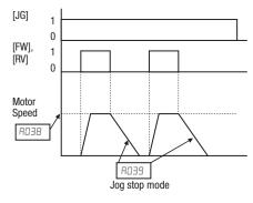
To enable the Run key on the digital operator for jog input, set the value 01 (terminal mode) in ADD2 (Run command source).
