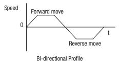
**Note** The MX2 can move loads in both directions. However, it is not designed for use in servo-type applications that use a bipolar velocity signal that determines direction.
