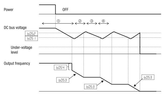
Should power be lost while the inverter is in run mode, this function will have the following effect:
