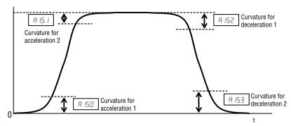
For use of EL-S curve be sure to use select multi-speed as frequency source to avoid nuisance change of frequency during acceleration and deceleration.
