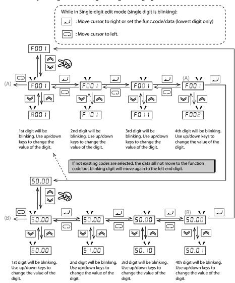
**Note** When pressing with cursor on the highest digit, the cursor will jump to the lowest digit. ((A) and (B) in above figure.)
