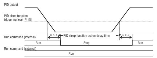
· PID Sleep function is always enabled, even the PID function is disabled.
