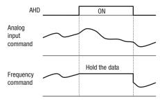
**Note** Set frequency remains when the inverter is switched with SET terminal with AHD on. Turn AHD terminal off to re-hold the set frequency.
