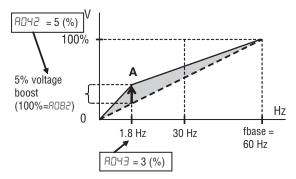
normal V/f ratio (shown at right). The function attempts to compensate for voltage drop in the motor primary winding in the low speed range.
