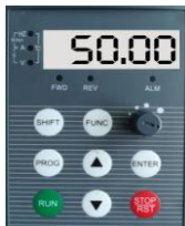
Fig 3-2 Stop Status Parameter Display Display Set Frequency "50.00"
