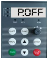
Fig 3-1 Power-on Parameter Display Initialization Display "P.OFF"
