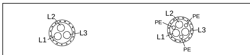
Figure 3-3 Recommended motor cables.
